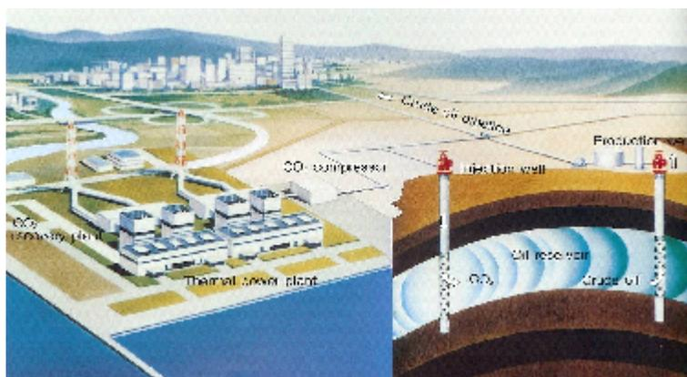
図 - 1 System of CO<sub>2</sub> - EOR(Enhanced Oil Recovery)
